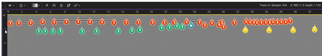
Figure 3 – GPR profile at a transition from the cut and cover conduit to a tunneled section near a tunnel portal.
