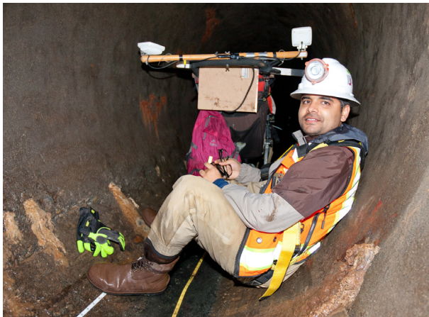
Figure 7. Shawn Spreng (upper left) during penstock inspection at Hyatt Power Plant shutdown, Oroville, CA, USA; Ashim Gajurel (bottom left) and Kush Chohan (right) facilitating tunnel diameter measurements and photo documentation during the San Pablo Tunnel inspection, San Leandro, CA, USA.
